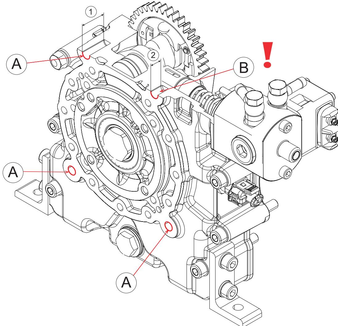
Specified tightening torque (MA) and screw-in depth:
