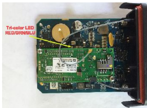
Figure 6: Status LED Location
